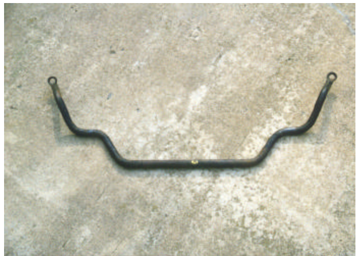
C9ZZ-E front sway bar paint marks: green to the left, yellow to the right.
